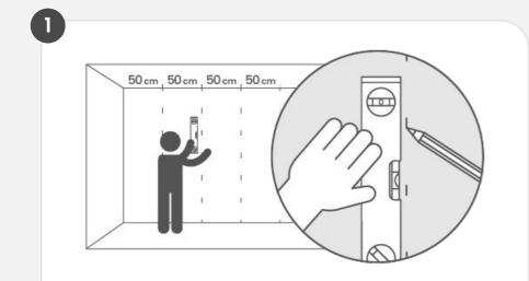
Using a spirit level and ruler, lightly draw vertical guide lines with a pencil where the wallpaper panels will be placed (every 50 cm).
