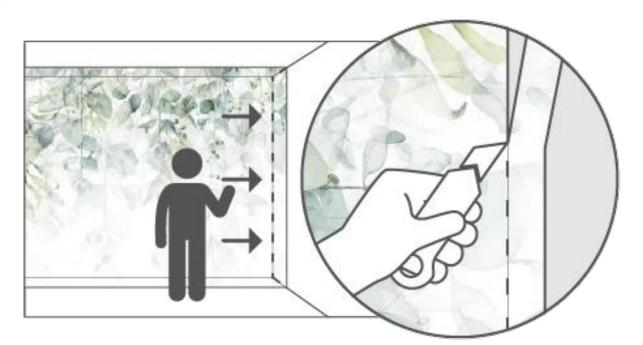
The last panel may need to be trimmed. If the ordered mural width is not a multiple of 50 cm, the final panel will be too wide and must be cut to fit the remaining wall space.
