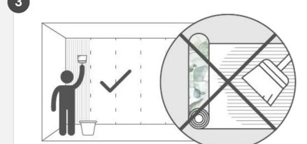
Apply a thin, even layer of adhesive directly to the wall using a brush (slightly wider than the panel).
