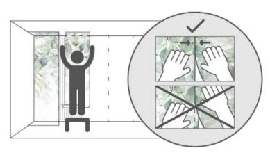
Repeat these steps for each additional panel. Continuously check that the panels adhere well and the pattern aligns (view from 1–2 meters away). The panels should not overlap.
