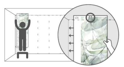
Start with the first panel. Identify the top side. Roll it with the print facing inward (starting from the bottom). Position the top edge of the panel against the glued wall, aligning it with the vertical line, and gently roll it down while pressing it to the wall.
