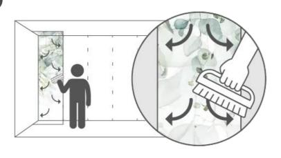
Remove air bubbles by gently smoothing the surface from top to bottom and from center to edges with a roller or wallpaper brush.
