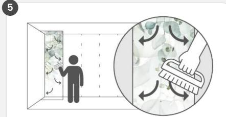
Remove air bubbles by gently smoothing the surface from top to bottom and from center to edges with a roller or wallpaper brush.
