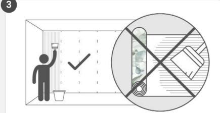
Apply a thin, even layer of adhesive directly to the wall using a brush (slightly wider than the panel).
