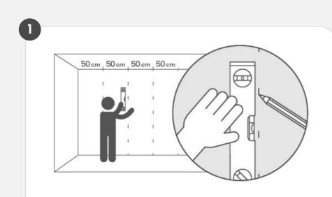
Using a spirit level and ruler, lightly draw vertical guide lines with a pencil where the wallpaper panels will be placed (every 50 cm).
