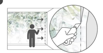
The last panel may need to be trimmed. If the ordered mural width is not a multiple of 50 cm, the final panel will be too wide and must be cut to fit the remaining wall space.
