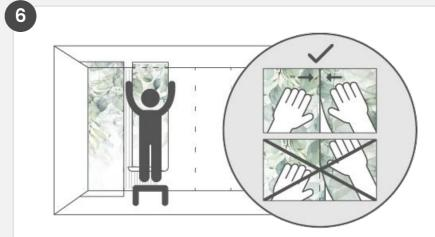
Repeat these steps for each additional panel. Continuously check that the panels adhere well and the pattern aligns (view from 1–2 meters away). The panels should not overlap.
