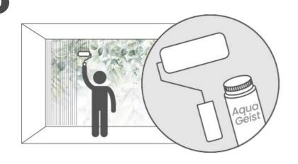
Apply the first coat of protective varnish using a foam roller – cover the entire surface carefully.
