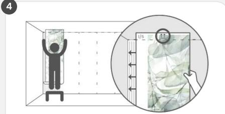
Start with the first panel. Identify the top side. Roll it with the print facing inward (starting from the bottom). Position the top edge of the panel against the glued wall, aligning it with the vertical line, and gently roll it down while pressing it to the wall.
